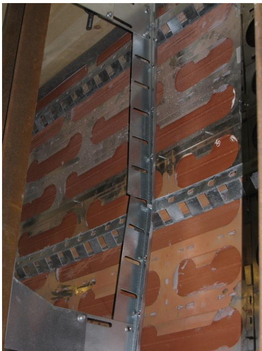
Photo 7. Deformed vertical rail after final failure.
